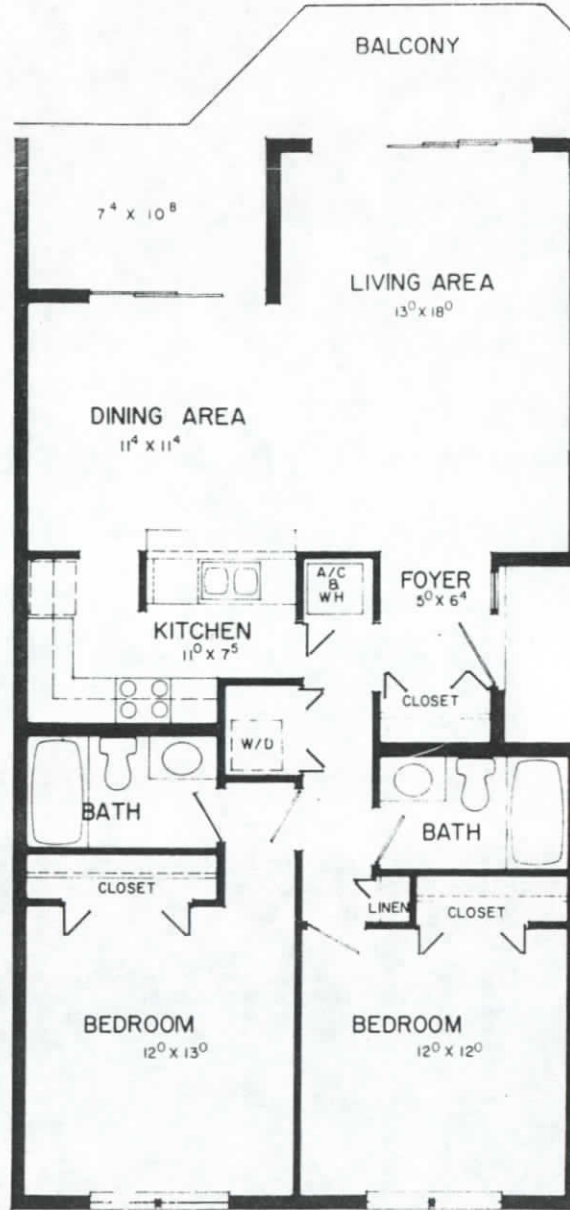
APARTMENT 4 - BUILDINGS C, E, F, H, J, L, N, Q, R - AS SHOWN APARTMENT 3 - BUILDINGS B, D, E, G, H, K, M, P, Q - REVERSE
